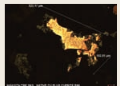
Below: Photomicrograph of typical Roseby native copper – a 0.322 millimetre long composite particle
