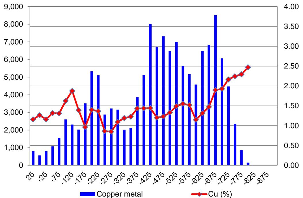
*Copper metal (left hand scale) and grade (% on right hand scale) in the Kylylahti mine mineral resource inventory in 25 metre vertical levels (RL). Copper metal in the resources is depleted by production to 31 December 2013.*
