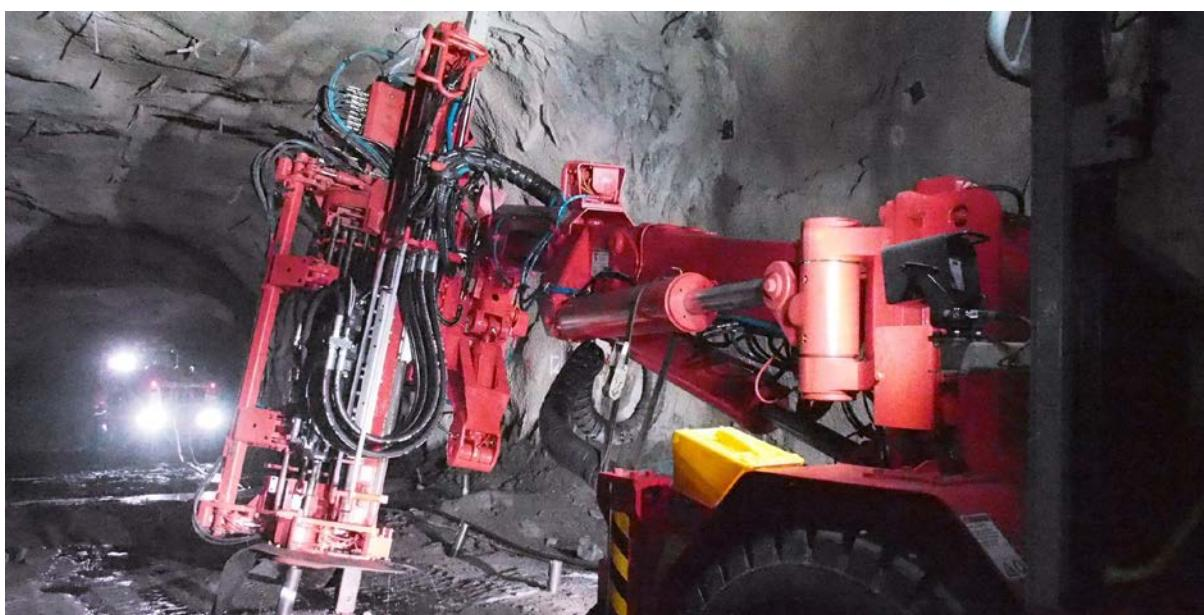
**Figure 2:** Production drilling at Kylylahti mine
