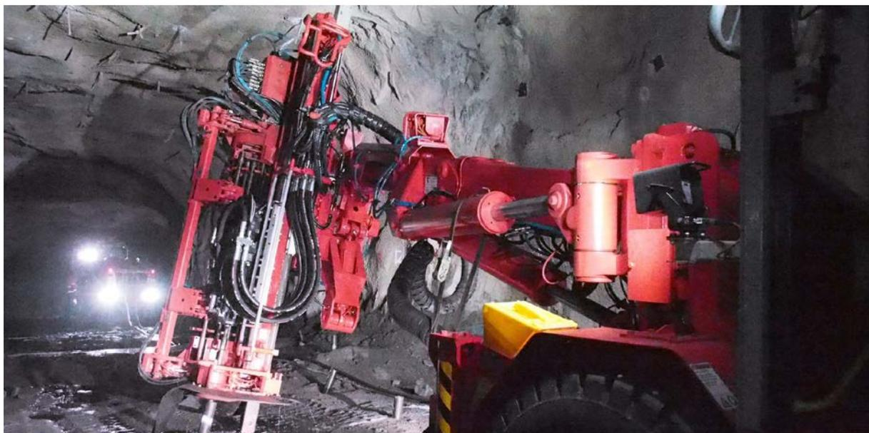
**Figure 2:** Production drilling at Kylylahti mine
