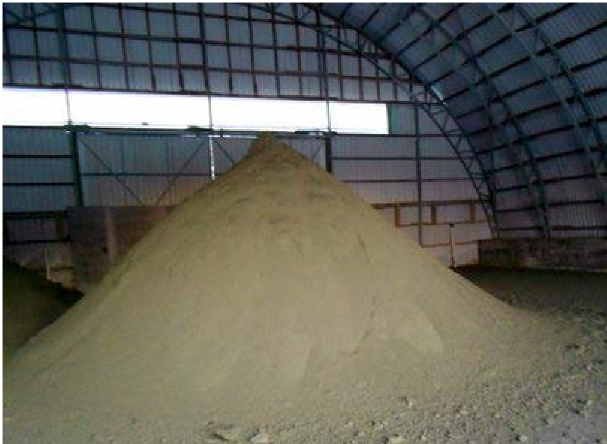
24% copper concentrate accumulating in the concentrate shed at the Luikonlahti processing plant
