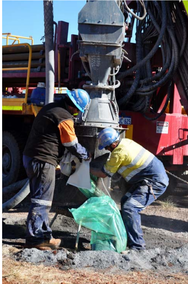
Collecting samples from RC drilling at Little Eva, Roseby Project. Swick Drilling have completed 20km of drilling this season
